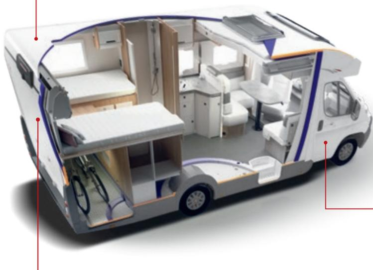
**WALLS.** External fibreglass, hail-proof, PVC frame and waterproof plastic inserts. High density perimeter protection in plastic: prevents any contact between inside and outside avoiding the inlet of water inside the walls. Fibreglass internal walls, resistant to humidity and free of thermal bridges that can be the cause of condensation or heat loss.
